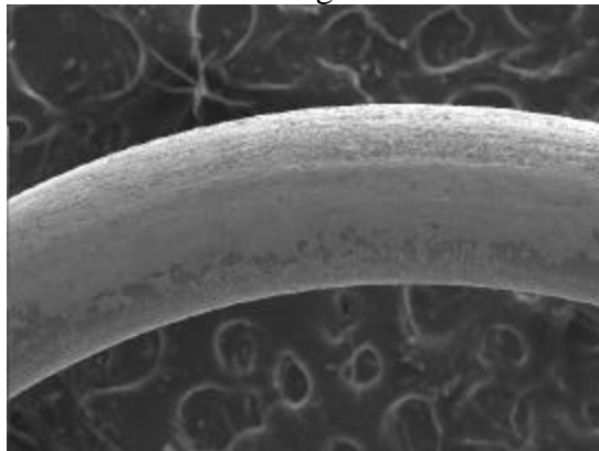
Figure 1: SEM micrograph of a DLC coated rhenium wire following a 90° bend test. The wire is 0.5 mm in diameter.
