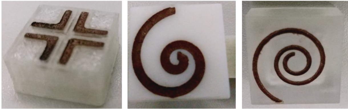
Fig. 1. a) Filled cross- phantom 2 mm channel, b) resolution phantom with exponential growing spiral layout and 2 mm channel width and c) 1 mm channel phantom with exponential growing spiral.
