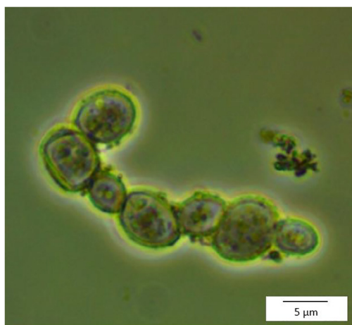
Fig. 3. Bright-field image of yeast cell modified with \text{Fe}_3\text{O}_4 particles and agglomerate of ferrimagnetic particles.
