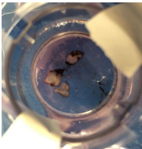
Fig. 10. Tissue samples in the cell plate after perfusion of MNPs, indicating severe agglomeration, possibly flocculation, in the tissue and on the bottom of the cell plate.
