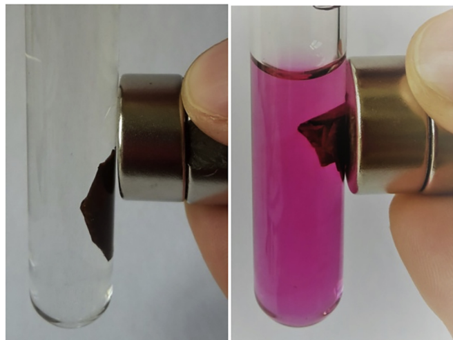
Fig. 8. Typical example of peroxidase-like activity of polyurethane nanotextile modified with chloroform-based MF leading to the formation of pink reaction product (oxidized DPD). Left – before the assay; right – after the assay.
