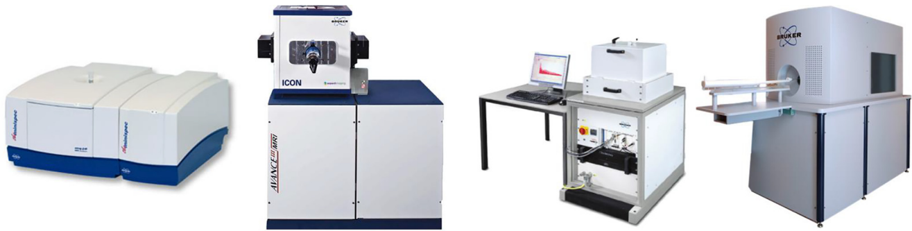
Fig. 1. Photographs of the used measurement systems: a) NMR relaxometer, Minispec mq60; b) Preclinical MRI, ICON; c) calibrated MPS device, MPS-3; d) Preclinical MPI scanner, 25/20 FF.
