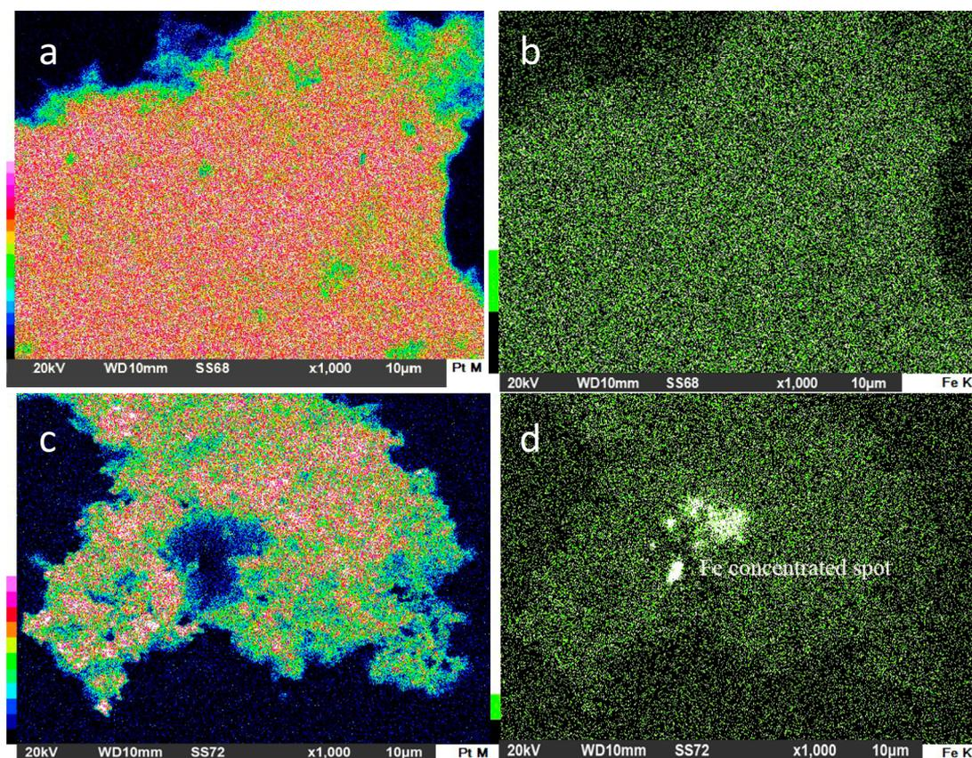
**Figure 2.** EDS mapping of a nonmagnetic Pt nanoparticle cluster (a, b) and a magnetic nanoparticle cluster (c, d) with the mapping of Pt (a, c) and Fe (b, d). The color differences are due to prolonged exposure.
