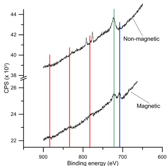
**Figure 1.** XPS spectrum of magnetic and nonmagnetic Pt (nano)particle clusters. Blue lines correspond to Fe 2p peaks, and red lines are Fe Auger peaks corresponding to peaks of oxides of iron; the green line represents the Pt 4s peak.
