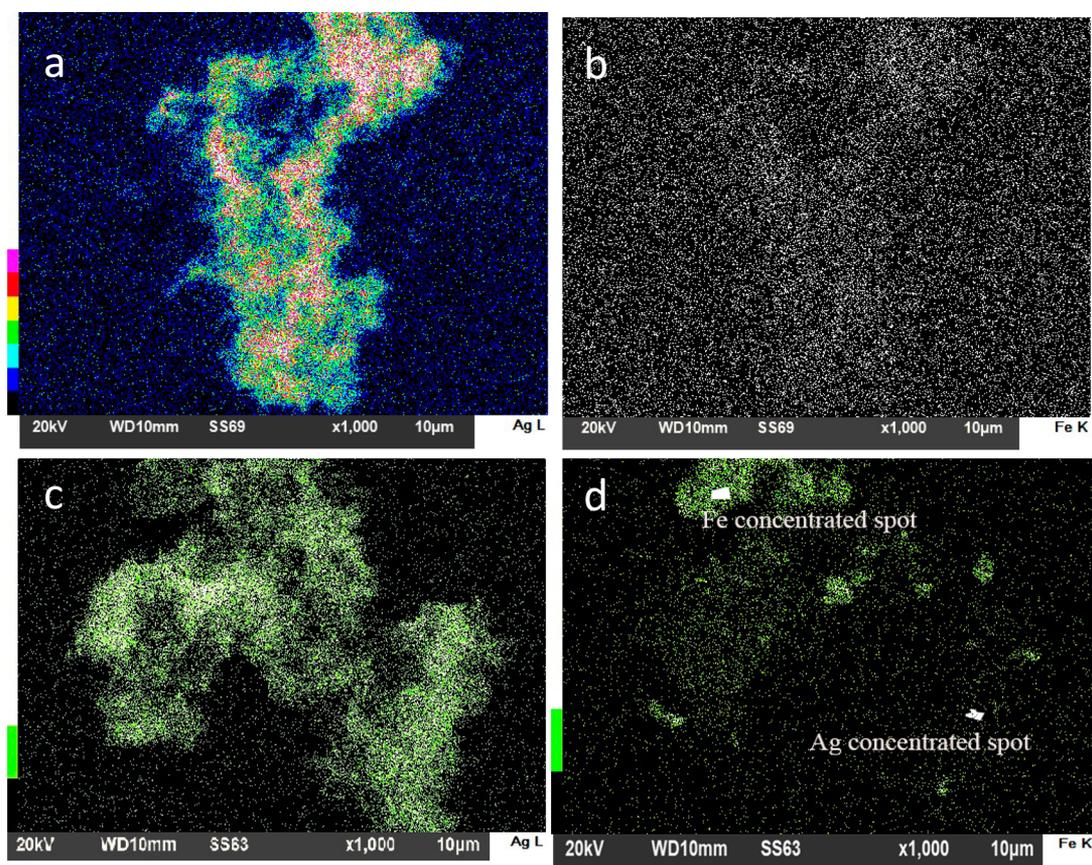
**Figure 3.** EDS mapping of a nonmagnetic Ag nanoparticle cluster (a, b) and a magnetic Ag nanoparticle cluster (c, d) with the mapping of Ag (a, c) and the mapping of Fe (b, d). Fe is insignificant in the nonmagnetic cluster, and in the magnetic sample it is concentrated in spots along the periphery of the NP cluster; the spots taken for point analysis are also indicated.
