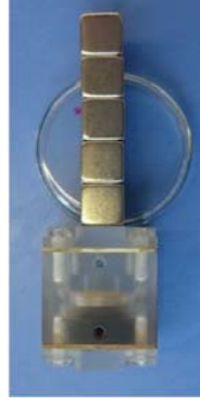
Two chamber system with mounted bar magnet for investigation of particles transport through different tissue of the eye.
