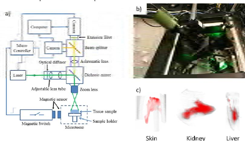
**Figure 1:** a) Schematic and b) photograph of the cryostat based co-registration 3D tissue imaging system. c) Sample measured magnetic nanoparticle distributions in skin, kidney and liver (fluorescent image only).
