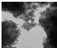
Figure 01. TEM micrograph of the nanoparticles of magnetite.
