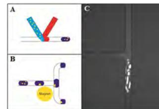
Fig.1. A Scheme of the droplet formation zone with magnetic particles and the sample mixture, B scheme of the magnetic splitter and the two daughter drops, C experimental image of the droplet containing magnetic particles inside the T-junction
