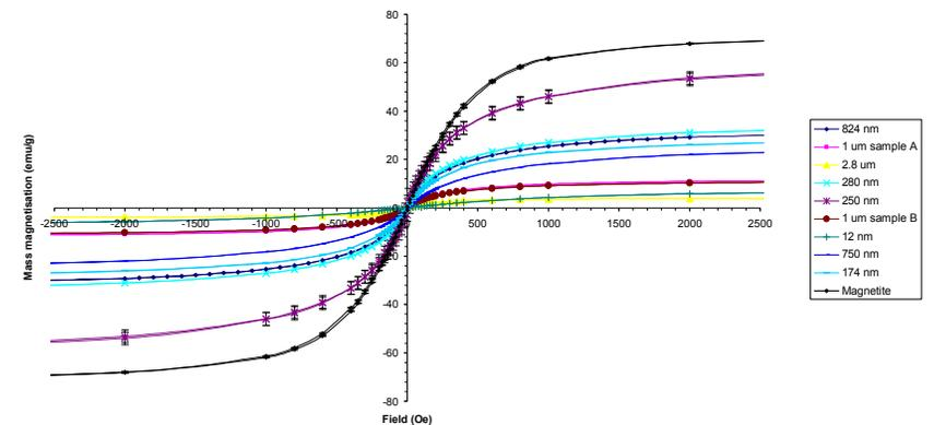
Commercially available particles saturate at fields greater than about 2000 Oe.
