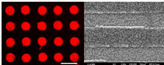
Figure. Both silicon wafer and GMR sensor were modified by APTES-Glu. After PAPP-A capture antibody, antigen, and biotinylated detection antibody binding, AF555-Streptavidin was added and bond to silicon wafer (left, scale bar is 400um), and 30nm streptavidin labeled nanoparticles was added and bond to GMR sensor (right).
