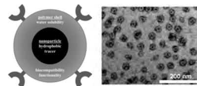
**Fig 1:** schematic concept of nanocontainer (left); TEM image of stained nanocontainers (right)
