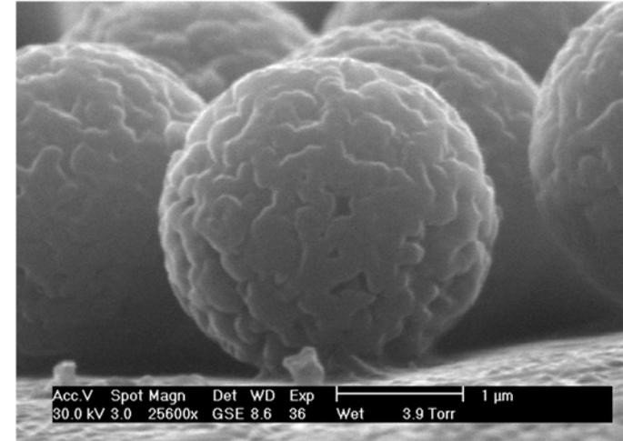
An EM image showing immobilised 2.8 μm-diameter particles on a plastic strip in a sandwich assay.
