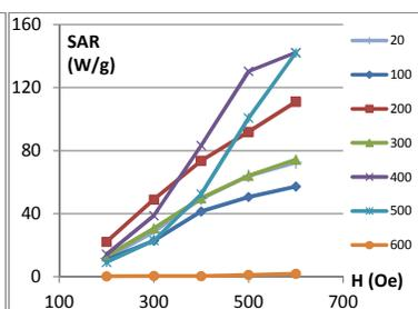
Figure 2. SAR of  $\text{Fe}^{II}_{1-x}\text{Co}_x\text{Fe}^{III}_2\text{O}_4$  MNP with  $x = 0.1$ , treated with  $20 - 600$  °C.
