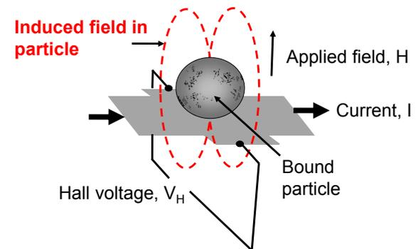
$$V_H = C (I \times H), \text{ where } C \text{ is a constant for the sensor}$$
