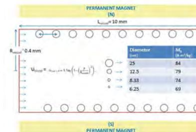
Schematic of the control volume used for studying the behavior of functionalized SPIONs as pharmaceutical carriers in magnetizable stent assisted drug targeting applications.
