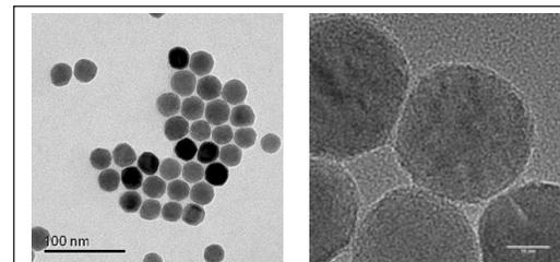
Figure 1. TEM (left) and high resolution TEM (right) of 27 nm diameter nanoparticles synthesized with this method. Scale bars are 100 nm and 10 nm respectively
