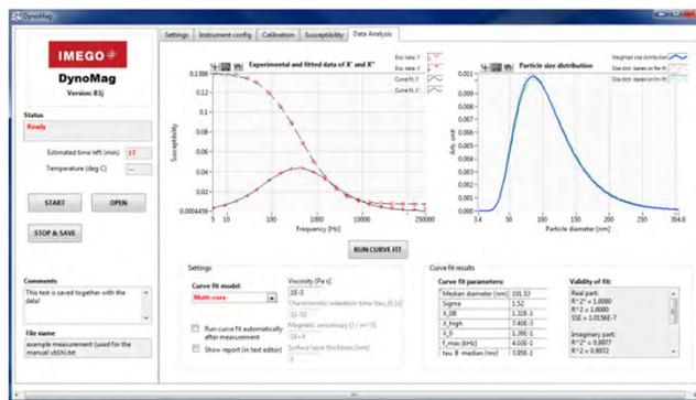
A fit to the measured data in the left figure. With the analysis package you can fit your experimental DynoMag data and determine the particle size distribution from the Brownian relaxation as well as Néel relaxation of single core particles.
