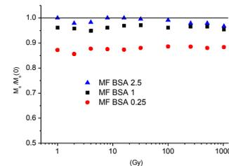
Dependence of reduced saturation magnetization on irradiation doses of water-based magnetic fluid containing magnetic particles coated with sodium oleate and modified with BSA. (The black line corresponds to value  $M_s(M)/M_s(0)$  of non irradiated sample).
