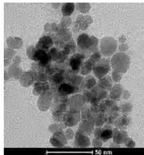
Figure – TEM image of SPIO NPs
