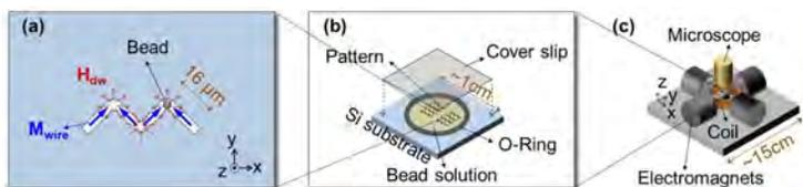
Schematic representation of: (a) Zigzag wires on Si platform with magnetizations  $M_{\text{wire}}$  pointing towards and away from vertices to create fields  $H_{\text{dw}}$  to attract magnetic beads to vertices. (b) Si platform with coverslip and O-ring to prevent fluid flow and evaporation. (c) Electromagnets and coil to generate fields in x, y and z directions. The platform is observed by a microscope.
