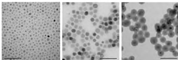
Examples of bare and silica coated cobalt-zinc ferrite nanoparticles possessing different size, the scale bar is 50 nm.
