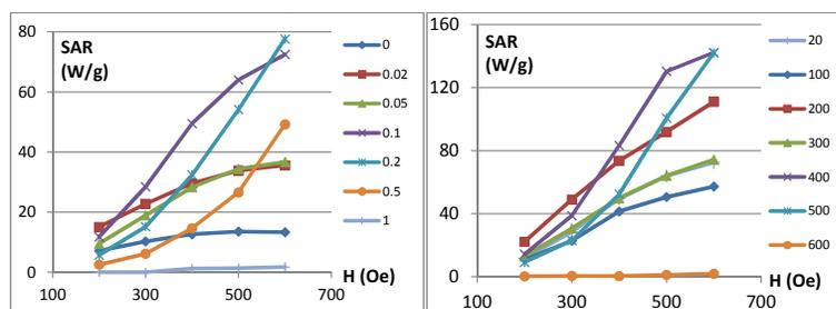
Figure 1. SAR of  $\text{Fe}^{II}_{1-x}\text{Co}_x\text{Fe}^{III}_2\text{O}_4$  MNP with  $x = 0, 0.02, 0.05, 0.1, 0.2, 0.5$  and  $1$ .
