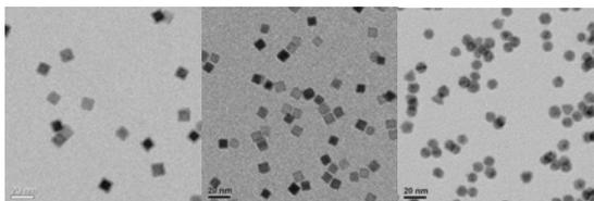
TEM images of Fe<sub>70</sub>Co<sub>30</sub>, Fe<sub>40</sub>Co<sub>60</sub> and Fe<sub>10</sub>Co<sub>90</sub> Nanoparticles
