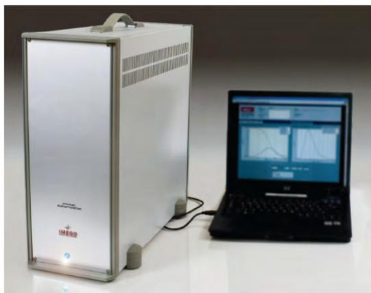
DynoMag is a portable, easy to use AC susceptometer. It measures the real and imaginary components of the AC susceptibility in a wide frequency range. The instrument enables determination of the magnetic properties of liquids, powders or solid samples.
