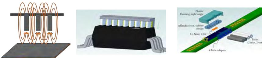
General diagram demonstrating the magnetic field from magnetic cilia on GMR sensor(Left). Vibration sensor on GMR SOIC package(Middle). Flow sensor/ actuator exploded view(Right)
