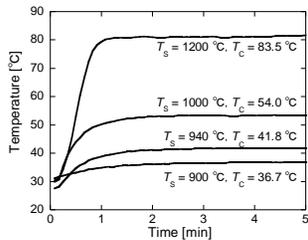
Fig.2 Temporal change of the suspension temperature under AC magnetic field.
