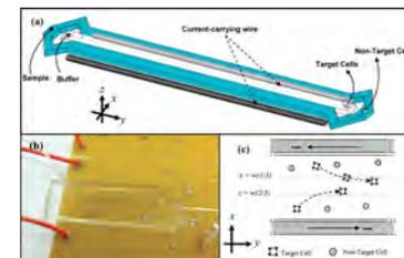
Figure 1. (a) Schematic illustration of the cell separation design. (b) Photograph of the microfluidic chip aligned on the electromagnet wire array. (c) Principle of magnetophoretic cell separation
