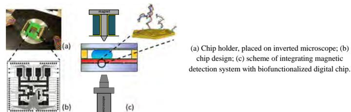
(a) Chip holder, placed on inverted microscope; (b) chip design; (c) scheme of integrating magnetic detection system with biofunctionalized digital chip.
