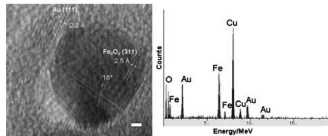
Fig 1. HRTEM image and EDX spectrum of a Fe<sub>3</sub>O<sub>4</sub>-Au NP
