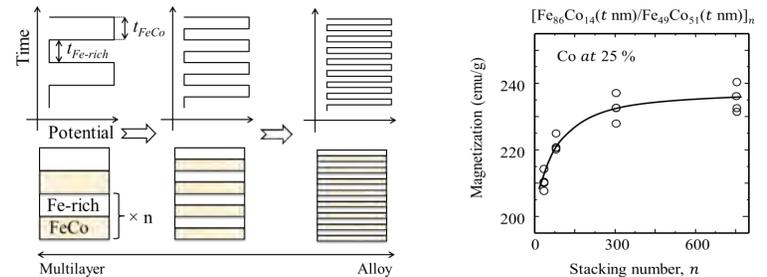
Fig. 1 Schematic of the pulsed-current and the corresponding nanostructure. The notation  $n$  outside the parenthesis denotes the stacking number.
