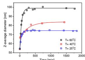
Figure 1: Adsorption kinetics of MFBSA8.0 (BSA/Fe<sub>3</sub>O<sub>4</sub> = 8.0w/w) at various temperatures.
