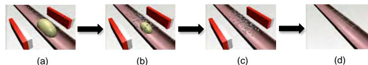
**Figure 1.** Schematic representation of lysis of an in-stent thrombus by injection and capture of tPA-nanoparticle conjugates at the stent surface under the influence of an external magnetic field (a-c). The nanoparticles are released after removing the magnets (d).
