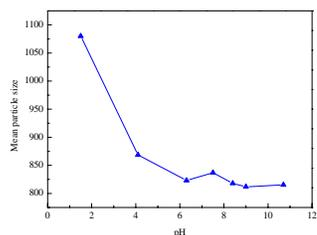
Fig. 1 The pH dependence of the mean particle size of  $\text{Fe}_3\text{O}_4/\text{P}(\text{AA-MMA-DMA})$  microspheres at 37 °C
