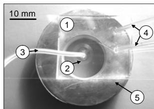
**Fig. 1:** Photograph of the microfluidic chip (1) showing the spiral structure (2), inlet (3), and two outlets (4). The octupole magnet (5) is visible beneath the chip
