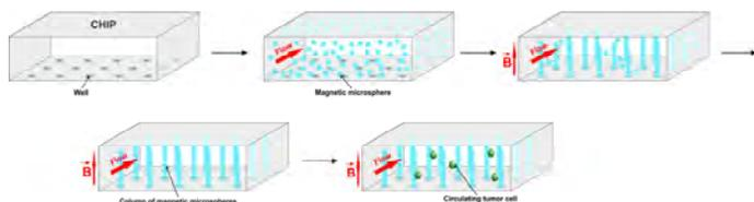
The Ephesia system. Allignment of magnetic microspheres into columns inside the chip under magnetic field and capture of epithelial cells.
