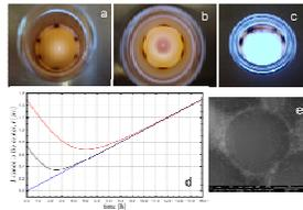
**Figure1.** Magnetophoretic behavior of a suspension of latex particles and SDS-NPs in water. (a) Initial mixture; (b) latex particles are concentrated in the center of the vessel forming a ring. (c) Both SDS-NPs and latex particles are trapped on the walls of the vessel. (d) Trajectories of the latex particles in the mixture at 60T/m. (e) SEM images in the backscattered detection mode of a sample extracted from the ring.
