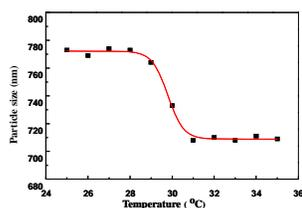
Fig. 2 The temperature dependence of the mean particle size of  $\text{Fe}_3\text{O}_4/\text{P}(\text{AA-MMA-NIPAM})$  microspheres
