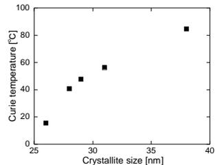
Fig.1 Curie temperature versus crystallite size for the synthesized particles.
