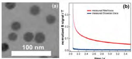
Fig. 1: (a) a typical TEM micrograph of LSCNPs and (b) Néel and Brownian relaxation traces of LSCNPs.
