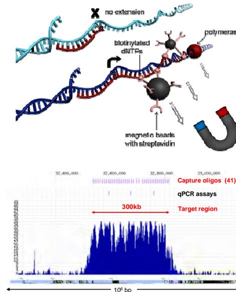
Region- and haplotype-specific extraction (RSE/HSE) is an automated, magnetic particle-based target enrichment method that captures large (10-40kb) segments of genomic DNA with high efficiency in a sequence- or SNP-specific way.
