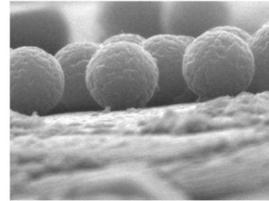
2.8 μm diameter particles
