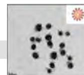
Fig.1 The TEM image of sunflower like  $\text{Fe}_3\text{O}_4/\text{Au}$  nanoparticles
