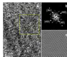
Fig. 1 HRTEM image of ferucarbotran nanocrystals (a); indexed diffraction pattern (b) and Fourier-filtered image (c) of the selected area viewed under the [233] zone axis.
