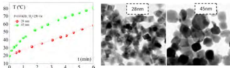
Figure 1. Variation of temperature with time for samples of different sizes at a set frequency of 110kHz and a field amplitude of 250 Oe.
