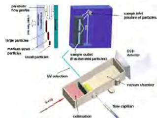
Separation of rod-like magnetic nanoparticle and online analysis with small-angle X-ray scattering
