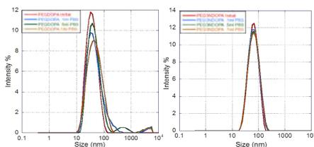
Figure 1: DLS intensity average of PEG DOPA coated particles and PEG TriNitroDOPA stabiles particles with increasing concentration of PBS
