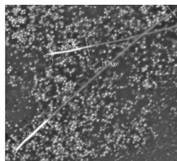
Fig 1: SEM image showing multilayers in two Gold/Nickel nanowires.
