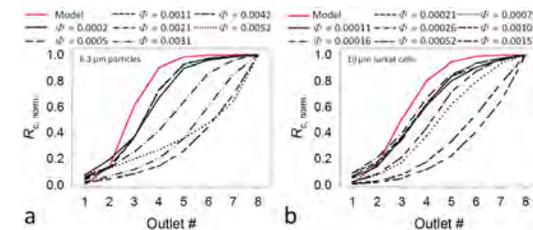
Figure. Normalized cumulative recovery of DMF fractionations with  $6.3 \mu\text{m}$  magnetic microparticles (a) and  $10 \mu\text{m}$  immunomagnetically labeled Jurkat cells (b). Data shown as cumulative mean recovery ( $n = 2$ ).
