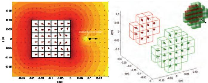
Figure 2. (Left) Optimal 36 element 2D push array. Brown arrows show optimal magnetization directions, colors indicate the resulting magnetic field strengths, and the black dot and arrow shows the push force at depth. (Right) Optimal geometry and magnetization directions for a 36 element 3D Halbach pull array. The optimal geometry is shown at top right, magnetization of the two layers is shown by red and green arrows for the back and front magnets.
