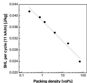
Dependence of the mass weighted specific hysteresis losses (SHL) on the packing density of magnetic nanoparticles measured at low field amplitude (11 kA/m).
