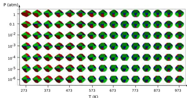
The shape map of hematite nanocrystals enclosed by surfaces  $(01\bar{1}2)$  (color-coded with green),  $(10\bar{1}4)$  (red),  $(10\bar{1}1)$  (blue, and  $(0001)$  (magenta). The pressure is of water vapor.
