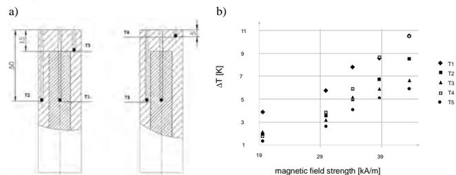
Figure 1a) Phantom with well-defined positions of the thermocouples named T1 to T5. b) Magnetic field dependence of the maximal temperatures for the different thermocouples.
