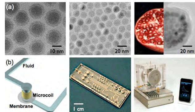
Figure 1. DMR (diagnostic magnetic resonance) platform. (a) Different types of magnetic nanoparticles developed for DMR assays. From left to right: Fe-based nanoparticles, Mn-doped ferrite, and multicore particles. (b) DMR system. From left to right: the schematic of an NMR probe, a microfluidic chip with integrated with NMR probes, and a portable NMR reader.
