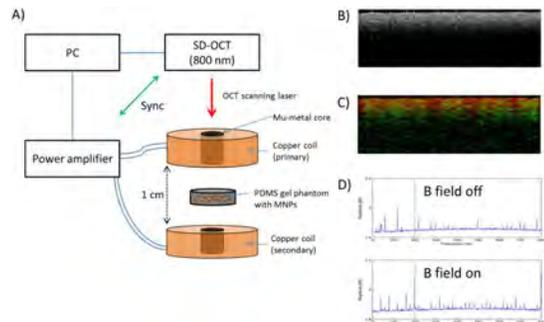
Figure 1. Schematic representation of the MM-OCT system: A) MM-OCT solenoid configuration, B) SD-OCT B-mode image, C) superimposed image of MM signal (green) and OCT B-mode image (red), and D) frequency spectrum (B field on /off) of MM signal.
