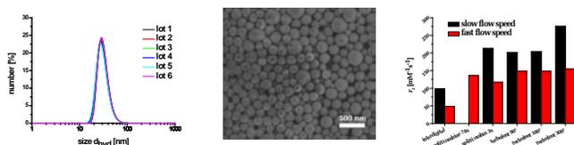
**Fig 1** – DLS measurement of 6 equivalent batches of single encapsulated particles (left), SEM image of 170 nm sized capsules filled with iron oxide particles (middle) and relaxivity  $r_2$  in dependence to flow speed and mixing chamber used during the phase transfer (right)
