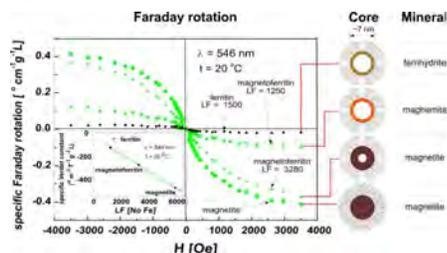
Fig. 1: Comparison of specific Faraday rotation for  $\lambda = 546$  nm as a function of the applied magnetic field for ferritin, magnetoferritins and magnetite aqueous suspension. The insert shows the dependence of specific Verdet constant on loading factor.
