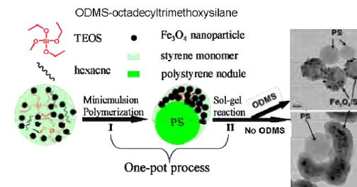
**Figure.** A novel one-pot colloidal reaction strategy is developed to synthesize Janus magnetic composite particles with high anisotropy, consisting of Fe<sub>3</sub>O<sub>4</sub>/silica inorganic hybrids and polystyrene nodule epitaxially arranged in a heterodimer morphology or capped shape.
