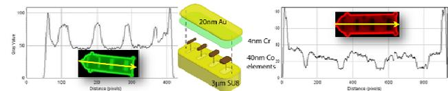
**Figure:** Exploded schematic of a hetero-functional magnetic microcarrier (centre) and line-intensity profiles showing microcarriers dual-labelled with fluorescein and TAMRA. The peaks and troughs are indicative of whether the fluorescence is on the top or bottom side respectively.
