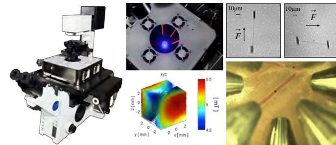
Left: The MiniMag system incorporated in an inverted microscope; middle: close-up of coils (top), simulation of magnetic field distribution for a field of 5mT along x (bottom); right: magnetic gradient based control of Ni nanowires (top) and NdFeB microspheres in blood vessels of a chicken embryo (bottom).
