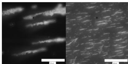
Figure 1: Dark Field Scattering for A) 550MW and B) 5000MW PEG coated 22nm nanoparticles under .1T external magnetic field
