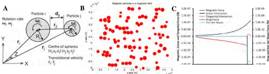
Figure A: Particle-particle kinematic variables; Figure B: Many particle simulation showing chain formation 100 $\mu$ s after starting with particles distributed at grid points. Figure C: Some of the forces acting between two particles. The reference particle is fixed in place while the particle under investigation is attracted by the magnetic force.
