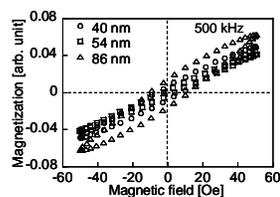
Fig. 1. Ac hysteresis loops measured at 500 kHz.
