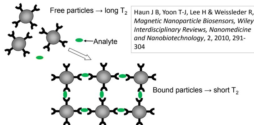
Clusters of cross-linked particles (diameter  $\approx 300\text{nm}$ ) decrease the transverse time constant  $T_2$  for the proton magnetic resonance of the water molecules. Unbound particles (diameter  $\approx 38\text{nm}$ ) have a smaller effect on  $T_2$ .
