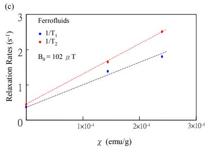
$1/T_1$  and  $1/T_2$  as a function of  $\chi$  in  $B_0 = 102 \mu T$ .
