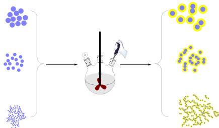
Scheme of assembly of magnetite clusters with different sizes in SiO<sub>2</sub> coating process
