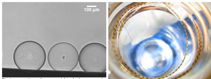
Giant magnetic polymer vesicles (polymersomes) prepared in a double-emulsion co-flows micro-chip.
