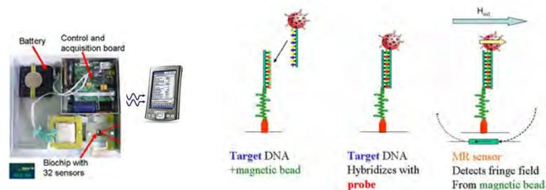
Prototype of the magnetoresistive chip-based platform & Biomolecular target-probe hybridization detection on-chip using magnetic labels as reporter system.
