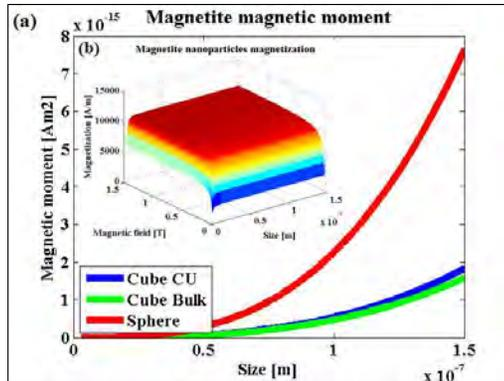
Fig 1: (a) Magnetic moment of magnetite particles for "Cube" and "Sphere" model. (b) Magnetization of biogenic nanoparticles with respect to particle size and magnetic field strength.
