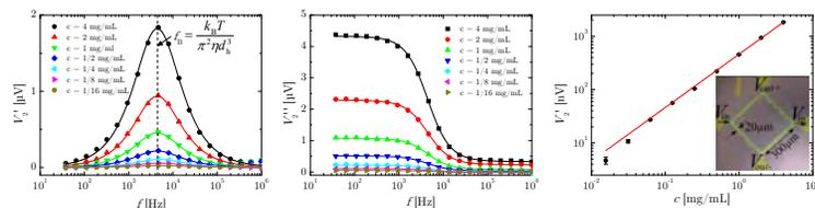
**Fig 1:** Second harmonic in-phase (left) and out-of-phase (right) sensor signals measured vs. frequency  $f$  for the indicated bead concentrations  $c$ . Signals are corrected using a background signal measured on a sample without beads. The solid lines are fits to the Cole-Cole model.
