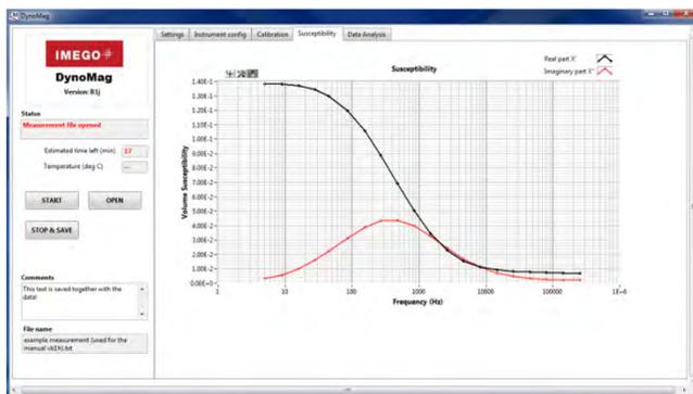
A DynoMag measurement of the AC susceptibility versus frequency for magnetic nanoparticles dispersed in a liquid (Chemical FluidMag cobalt-ferrite). The decrease in real part and the maximum in imaginary part of the susceptibility around 400 Hz is due to Brownian relaxation of the nanoparticles. The residual non-zero real susceptibility above 10 kHz comes from fast Néel relaxation.
