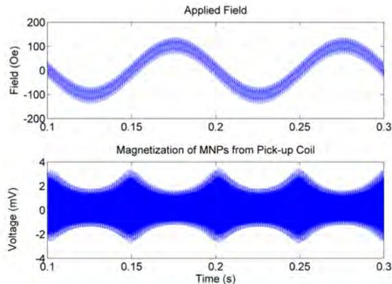
Signal from pick-up coil is digitized and recorded in time domain. The applied field (top) contains low frequency 10 Hz and multi-tone high frequencies (1 kHz, 5 kHz, 10 kHz, 15 kHz, and 20 kHz). The magnetization of MNPs (bottom) shows the periodic nonlinear response.
