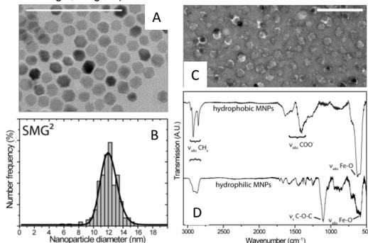
Figure. Bright field TEM-image (A) and corresponding histogram (B) of SMG<sup>2</sup> MNPs. The histogram, plotted as diameter versus number frequency, was fitted with a lognormal curve. Background stained bright field TEM-image (C) of poly-ethylene glycolated silane functionalized MNPs. The FTIR-spectra (D) of MNPs before and after silane functionalization. Scale bar of the TEM images is 100 nm.
