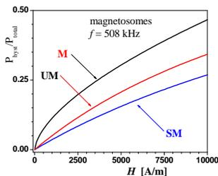
**Fig. 1:** The contribution of hysteresis processes to the total release of thermal energy for the three samples (M-normally isolated, UM-after ultracentrifugation, SM-after sonification) as a function of magnetic field strength.
