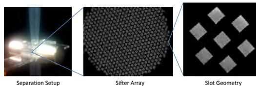
Figure 1. Magnetic Sifter Assembly
