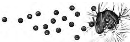
Figure 1: Schematic representation of the impact of thermal neutrons on iron-boron nanowires with the resulting highly energetic \alpha and ^7\text{Li} particles heading for a tumor cell
