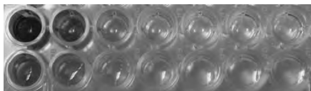
Figure 1: bacterial magnetic nanoparticles show intrinsic peroxidase-like activity. The top row samples catalysed the reaction of the peroxidase substrate 3,3,5,5-tetramethylbenzidine (TMB), the bottom row of samples catalysed the reaction of the other peroxidase substrate o-phenylenediamine (OPD). The samples left to right show decreasing magnetic nanoparticles concentrations.
