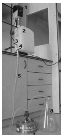
Fig. 1. Flow-through magnetic separation system. 1 – mechanical overhead stirrer; 2 – container; 3 – valve; 4 – screw clamp; 5 – tubing; 6 – bottle; 7 – Sepmag Q magnetic separator; 8 – bottle for collection of magnetic particles depleted solution
