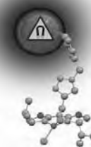
Schematic representation of a chiral ligand/transition metal- complex covalently grafted on magnetic Co/C-nanoparticles.
