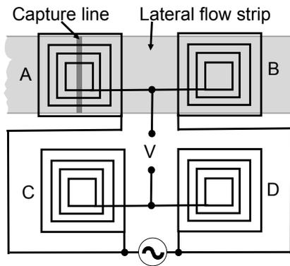
A, B, C & D are identical coils connected in a bridge circuit. A & C are wound in opposite direction to B & D. The lateral flow strip does not move and coil A is positioned over the capture line.
