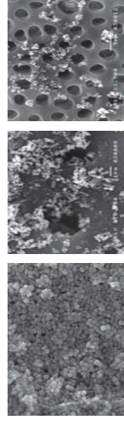
FE-SEM images of (A) magnetic nanocubes, (B) front and (C) back of FMNCs/PDMAEMA infiltrated through dentin disc.
