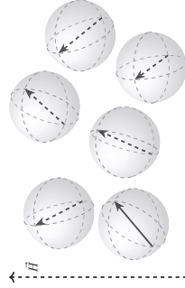
Figure 1: Damped precession of magnetic moments of MNPs in random positions and orientations due to an external magnetic field, H .
