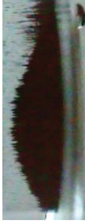
Figure In-situ observation of deposition of magnetic particles on the ferromagnetic filter under 10 T
