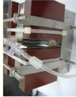
Schematic representation of the specific magnetic column for high cell sorting efficiency
