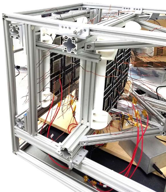
**Fig. 6.** Arrays of electropermanent magnets have been developed for magnetic resonance imaging and particle manipulation.
