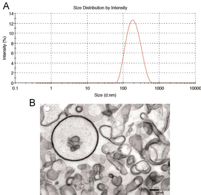
**Fig. 3.** (A) Size distribution of the MNE/CIAIPc sample assessed by photon intensity scattering analysis revealing average size of 173.6 nm and polydispersity index of 0.174. (B) Morphological analysis of the nanoemulsion/chloroaluminum phthalocyanine sample at 0.025 mg/mL using high-resolution TEM images recorded at 70 kV (44,000 $\times$ ).
