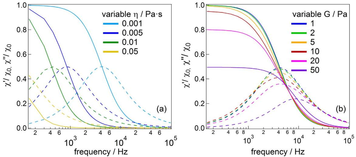
**Fig. 1.** Simulated ac susceptibility spectra (real part:solid lines, imaginary part:dashed lines) based on Raikher model: (a)  $G=0.1$  Pa,  $\eta$  varying between  $10^{-3}$  Pa·s and  $5 \cdot 10^{-2}$  Pa·s (b)  $\eta=10^{-3}$  Pa·s,  $G$  varying between 1 Pa and 50 Pa.
