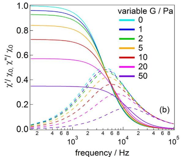
Fig. 2. Simulated ac susceptibility spectra (real part:solid lines, imaginary part:dashed lines) based on modified Debye model: a)  $G=0$  Pa,  $\eta$  varying between  $10^{-3}$  and  $1 \cdot 10^{-1}$  Pa · s b)  $\eta=10^{-3}$  Pa · s,  $G$  varying between 0 and 50 Pa.
