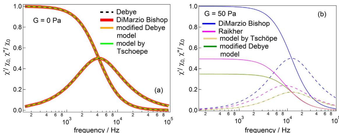
Fig. 3. Comparison of ac susceptibility spectra based on the models Debye, DiMarzio Bishop, modified Debye model, model by Tschöpe for (a)  $G=0$  Pa and additional with Raikher's model for (b)  $G=50$  Pa.
