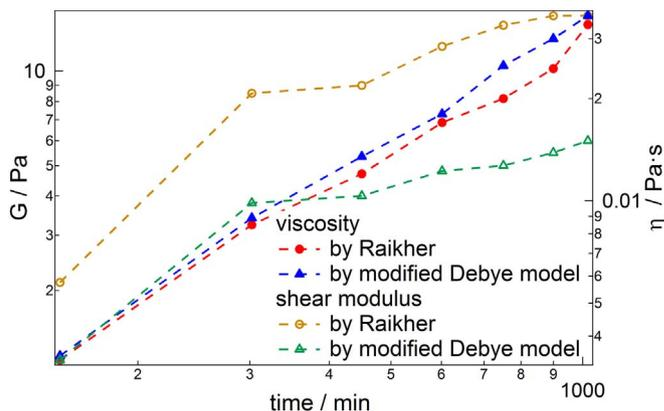
Fig. 5. Viscosity (closed symbols) and shear modulus (open symbols) determined by the models of Raikher and modified Debye model for a 2.5 wt% aqueous gelatin solution sample.
