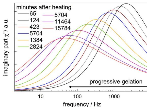
Fig. 4. The imaginary part of the ac susceptibility spectra measured on the 2.5 wt% gelatin solution.
