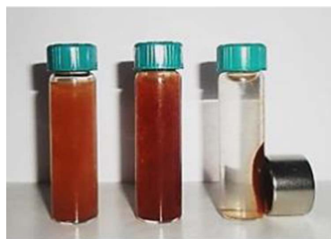
Fig. 5. Appearance of native Leptothrix sheaths suspension (left), suspension of sheaths after magnetic modification (middle) and demonstration of magnetic separation of magnetically modified sheaths (right). Almost the same appearance was observed after magnetic modification with microwave synthesized magnetite particles and with magnetic fluid.
