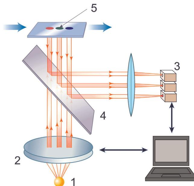
Fig. 1. Optical scheme of the spectral correlation interferometry: 1 – radiation from a superluminescent diode, 2 – scanned Fabry–Perot interferometer, 3 – photodetectors, 4 – beam splitter, 5 – biochemical reactions on the surface of a cover slip.
